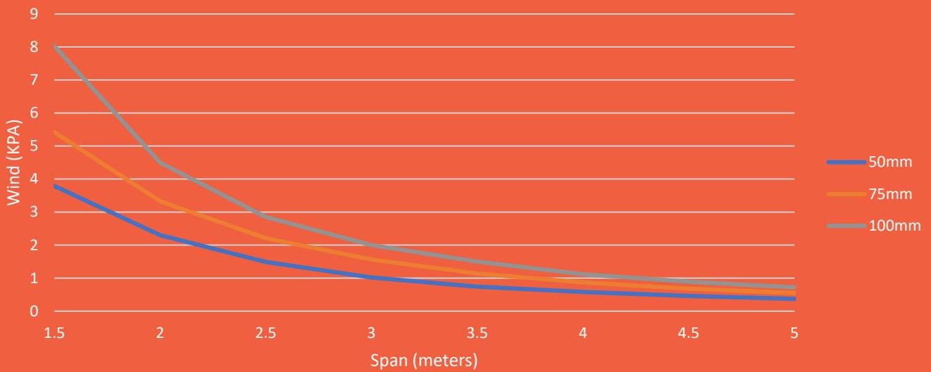
**NOTES:** Self-weight of the panel has been allowed for, plus an allowance of up to 10kg/m<sup>2</sup> for light duty fittings (lights, etc.). No other dead loads permitted. Pressures specified are for wind gusts only per AS/NZS 1170.2
